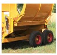
Optional Additional Axle: Adding an axle minimizes the tongue weight and makes it more stable, especially when backing on a trailer. (Highway tire only)
