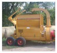
3-Foot, 80-Degree Enclosed Curved Spout: This spout can be rotated 360 degrees with the in-cab joystick control which can easily allow you to position the desired amount of product anywhere you want. It also has attachments that will allow you to direct your material and blow through a 10" hose
