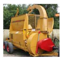
Blower/Fan: The fan in the blower has replaceable fins and shafts that can be replaced without removing the blower from the machine. The 2574 has three spout options which do the jobs of cattle feeding and bedding, and also erosion control.
