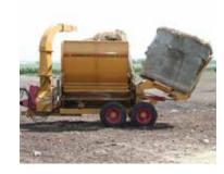
Two-Stage Bale Loader: Haybuster's single-cylinder two-stage loader makes it simple to load a bale into the chamber. A second bale can also be carried on the loader to expedite the job.
