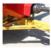
Centering hitch: Versatile hitch that positions machine directly behind tractor for transport and loading on trailer.
