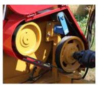
4-Groove Belt Drive System: 1000 RPM PTO drive through a set of 4-groove belts that drive the fan and rotor. With belts, the 2574 becomes more durable and smoother with less maintenance
