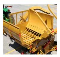
Bale Chamber: Complete with the 3-chain slat conveyor that has been an exclusive feature with Haybuster for many years, the 2574 is now available with 1 ¼" drive shafts, bearings and heavyduty chain. The chamber is taller to accommodate today's bigger bales. Nine slugbars hold the bale at bay from the rotor and are easily adjustable to get the product size you need.
