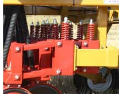
**Down Pressure System:** Each linkage has simple down-pressure adjustments from 135 lbs. for conventional seeding up to 300 lbs. for no-till application.
