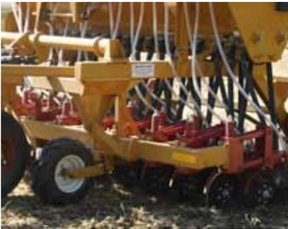
**7" Row Spacing:** All Haybuster drills plant with 7" spacing and each linkage is offset 9 ½" for planting in heavy residue.
