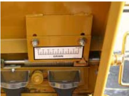
**Infinite Seed Rate Adjustment:** Easy to set, each box has infinite seed adjustment for accurate seeding rates, no matter what seed you're planting.
