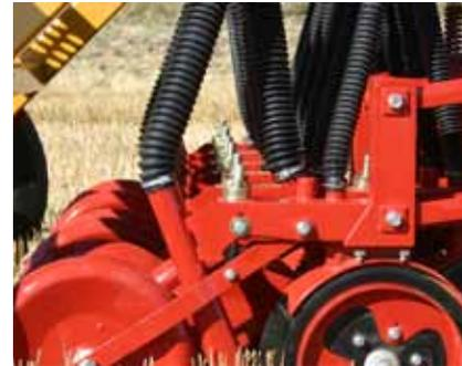
**Depth Control Adjustment:** Simple, solid depth control adjustment on each linkage.
