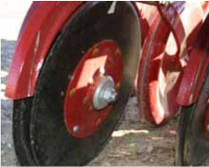
**Lead Coulters System:** Lead coulters blade is offset 1 ½" in front of dual disc, allowing for cutting of trash and penetrating the soil.
