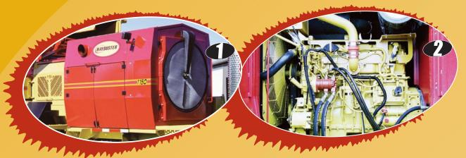
The enclosed engine compartment and rotary screen protects the engine from dirt and debris buildup. A covered engine also reduces the noise level. AND the 1150-1155 gives you easy access to the engine with a 3-door entry on both sides, plus a front door to the radiator.
